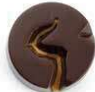
» Yuvarlak Çatlak Round Crack
